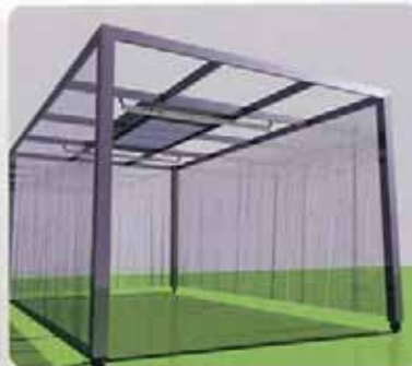
Installed height from target: 150mm Use of FFU laminar flow F-10 Frequency setting: 1Hz d-48 Pulse ratio setting: 48%
