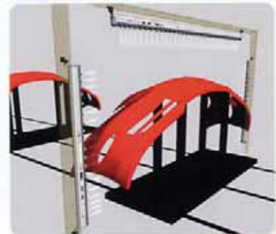
Installed height from target: 500mm Air pressure: 0.5MPa F-30 Frequency setting: 3Hz d-50 Pulse ratio setting: 50%
