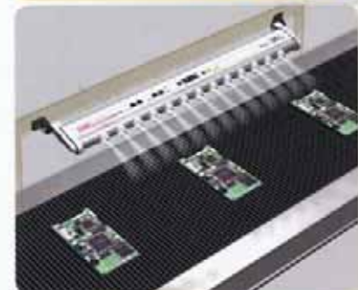
Installed height from target: 200mm Air pressure: 0.1MPa F-20 Frequency setting: 20Hz d-51 Pulse ratio setting: 51%
